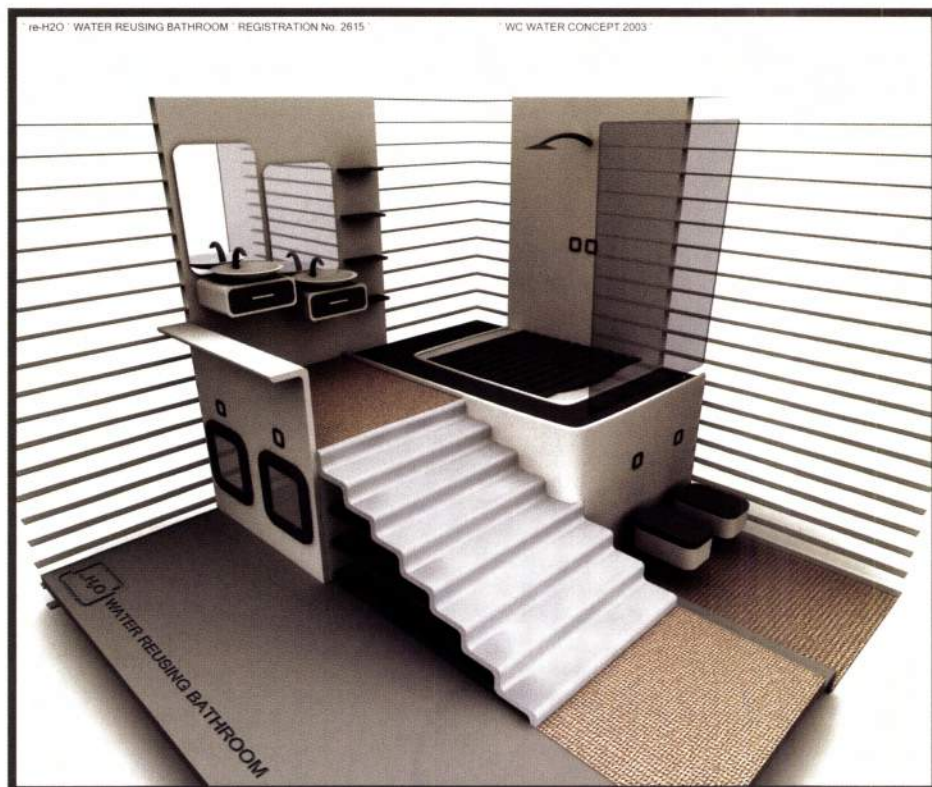
Kúpeľňa Re-H 2 O šetrí vodu. Odpadová voda zo sprchy, práčky či umývadla sa zbiera v cisterne. Zbaví sa nečistôt a použije sa na splachovanie záchoda / Bathroom Re-H 2 O - water reusing bathroom. Sewage water from sinks, shower and washing machine is collected into a cistern. After that, it is cleaned from the biggest dirt and used to flush the WC.
