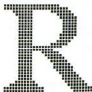
Simplified, diagrammatic representation of a digitized character. The two sizes are both constructed to the same resolution. The bigger the size the more pixels are available to draw the shape so the definition can be more detailed.
